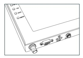
BNC – Composite Input VGA – Video Graphics Array DE15 Connection HDMI – High-Definition Multimedia Interface Input Connection Power Port – 12-24v Input
