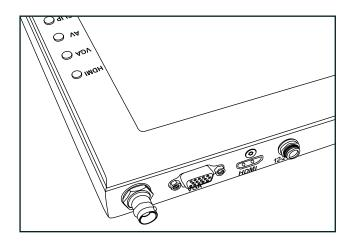
BNC – Component Input VGA – Video Graphics Array DE15 Connection HDMI – High-Definition Multimedia Interface Input Connection Power Port – 12-24v Input
