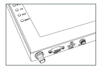
BNC – SDI Input VGA – Video Graphics Array DE15 Connection HDMI – High-Definition Multimedia Interface Input Connection Power Port – 12-24v Input
